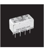
The .150 Grid relay, the smallest (.320 inches high) 2 Amp rated relay available in commercial and military qualified models, is now available in the long life version. Capable of over 100,000,000 mechanical operations at low level and signal load, the .150 Grid relay provides the simplicity of relays for circuit design, the low circuit resistance of precious metal contact systems, and the long life processing that has made CII relays the standard for guality and reliability.
